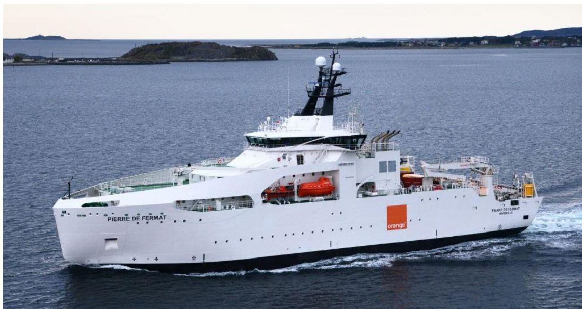
Figure 8: Navire câblé (source : Orange Marine)
